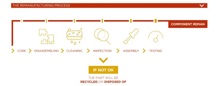
Once delivered, cores are disassembled, cleaned, and inspected. After inspection, all unrecoverable parts are recycled or disposed of. Strict adherence to current laws is guaranteed throughout the process with regard to the proper disposal of products or parts that are no longer usable and thus discarded.
